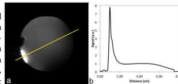
Figure 3. (a) An image acquired with both the 16-channel whole-brain coil and 7-channel chamber coil active. (b) The resultant signal profile.
